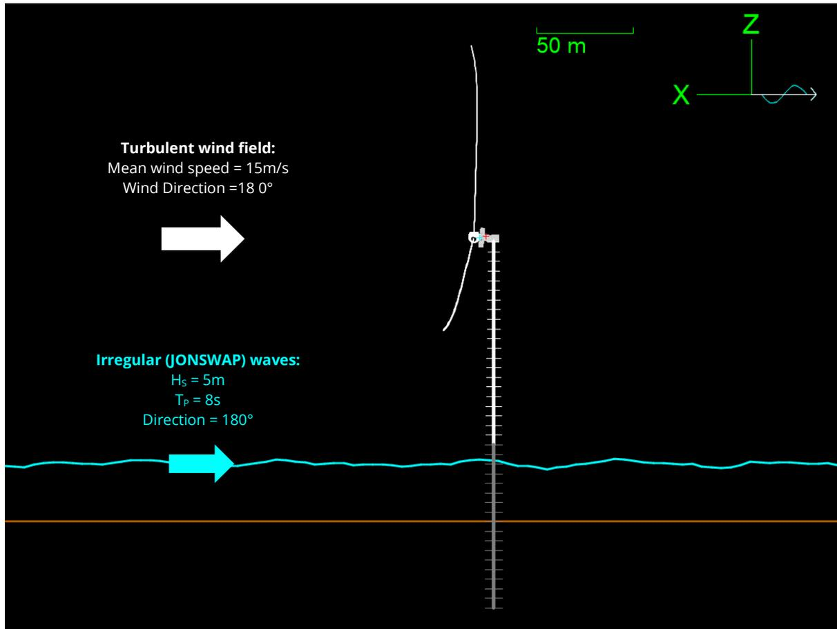
On the *wave calculation* page of the environment data form, we have specified a *wave kinematics cutoff depth* of 30m. This is measured downwards from the mean sea surface, and, below this depth, the wave kinematic fluid velocity and acceleration are taken to be zero. The default value here is *infinity*, which is equivalent to not having a cutoff depth at all.
