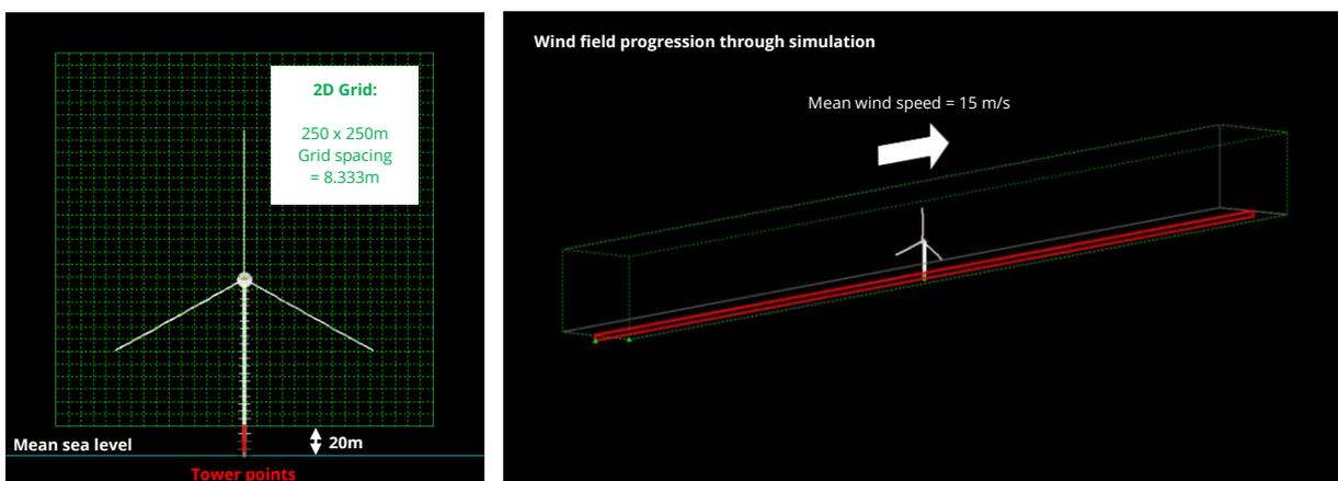
The *file header* also reports some information about the tower points included as part of the .bts file. As the bottom of the 2D grid is positioned 20m above the sea surface, the tower points help to ensure wind loads are received by the length of tower between the grid and the sea surface.
